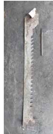
This is the equipment used to help cut ice as part of the local harvesting business.
