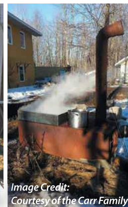
Tucked into a car shelter to get it out of the weather. Hank Carr says he watched a lot of YouTube videos and looked at a lot of designs before building his system. He uses tubing and a reverse osmosis system to increase the amount of sap he gets from his trees.
