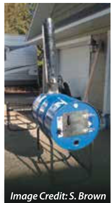
Inspired by memories of helping his grandparents make maple syrup S. Brown's teenage son built an evaporator from a re-purposed fuel drum, the metal frame of a generator and an exhaust pipe from a truck.
