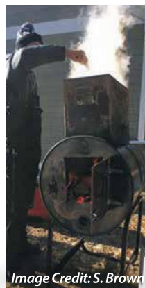
Inspired by memories of helping his grandparents make maple syrup S. Brown's teenage son built an evaporator from a re-purposed fuel drum, the metal frame of a generator and an exhaust pipe from a truck.
